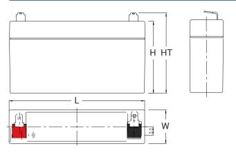
**L**: 3.81 (97) **W:** 0.94 (24) **H**: 2.02 (51.5) **HT**: 2.26 (57.5) Tolerances are +/- 0.04 in. (+/- 1mm) and +/- 0.08 in. (+/- 2mm) for height dimensions.
